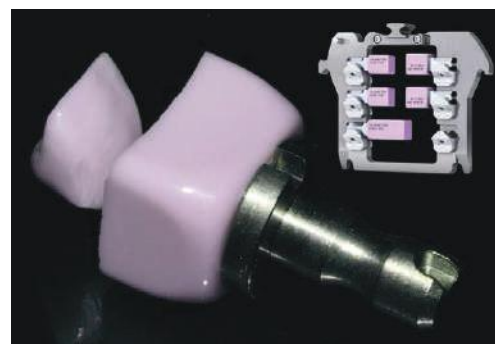
08 - Lithium disilicate block (IPS e.max CAD) in the blue intermediate crystalline stage on the e.matrix holder (for the Zenotec select milling machine) ready for wet machining
